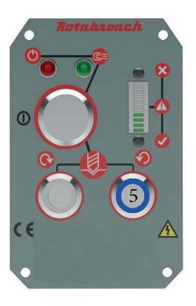
1. Ensure power to the machine, red LED will illuminate (1).
