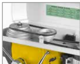
Upper cover opening with safety microswitch
