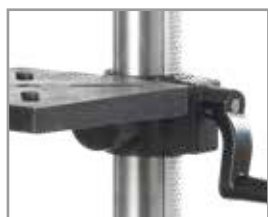
Workbench height adjustment thanks to a rack
