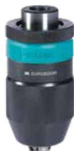
Drill chuck quick connect DIA Ø 1.5 - 13 mm 1/2" x 20 UNF connection Keyless IBQ.13
