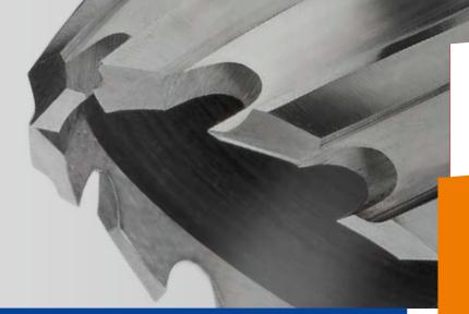
Euroboor HSS-Cobalt annular cutters are made of Molybdenum-Chromium-Vanadium-Tungsten alloy High Speed Steel with an additional 8% Cobalt (M42). The HSS-Cobalt annular cutter is specifically designed to remain cool when cutting holes. All flutes are fully ground, resulting in super-fast feed rates and smooth holes
